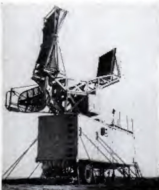
"Volscan" radar truck and antenna are hundreds of yards from control room, right, in underground bunker
